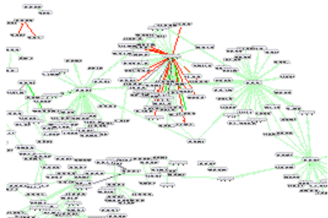
Figure 8 : Red lines show heavy traffic and could be a potential cause of a network slowdown; whereas light green illustrate a negligible amount of traffic between nodes.
